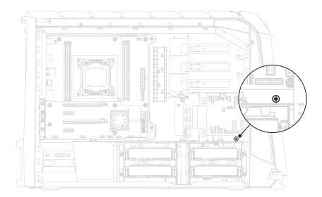
Remove the screw that secures the right-side top panel.
